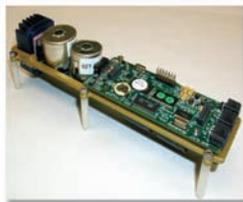
*Micro-Modem motherboard (inset). Conceptual diagram of sensor-modem network. Message relay will increase ranges beyond the direct path limit.*
