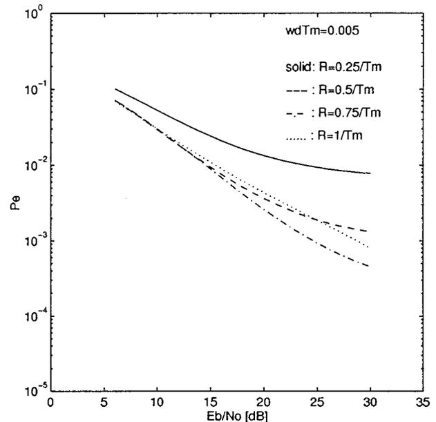
FIG. 4. Single-channel QPSK performance for varying symbol rates.
