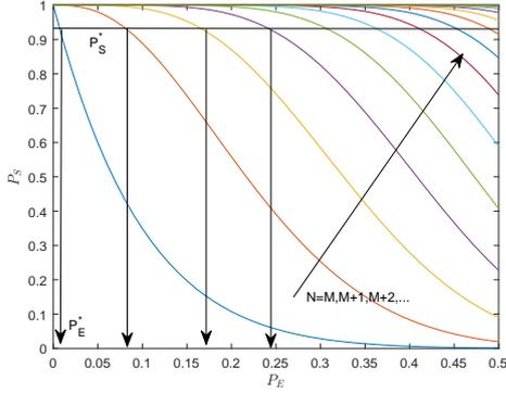
Figure 1: Probability of successful decoding vs. probability of packet error for different values of  $N$ .
