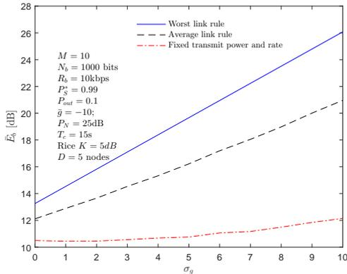
(c) Average energy per bit as a function of the channel fading parameter  $\sigma_g$ . As seen in *Case 1*, higher savings are available when the channel fading increases.
