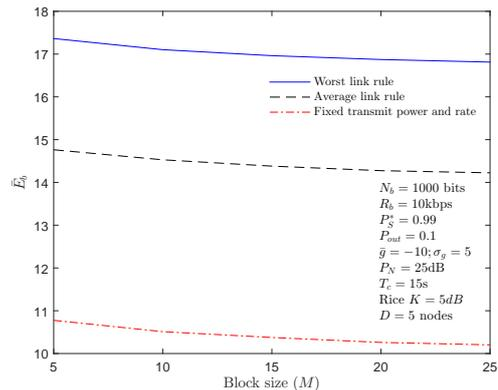
(a) Average energy per bit as a function of the block size  $M$ . Although larger blocks are favorable as they lead to lower average energy per bit, it is important to keep in mind that the block fading model should not be violated.
