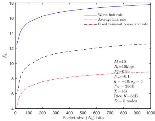
(b) Average energy per bit as a function of the packet size  $N_b$ . Although smaller packets lead to lesser average energy per bit, design choice for should also consider the average throughput.
