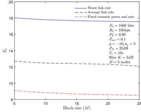
(a) Average energy per bit as a function of the block size  $M$ . As in *Case 1*, larger block sizes are favorable as long as they do not violate the block fading assumption.
