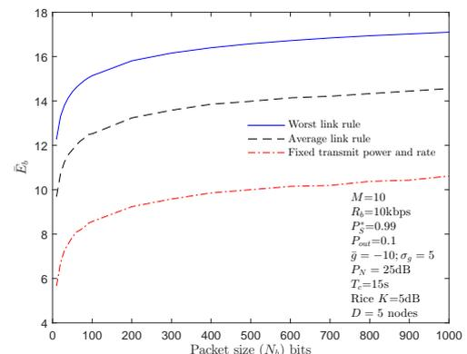
(b) Average energy per bit as a function of the number of bits in each packet. Although smaller packets use less energy per bit, the average throughput will suffer with smaller packet sizes.
