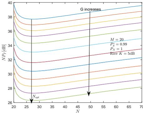
Figure 2: Plot of  $NP_T^*$  vs  $N$ . To minimize the average energy per bit, the number of coded packets and the transmit power should be chosen such that the product  $NP_T^*$  is minimized (subject to system constraints  $P_{T,max}, N_{max}$ ).
