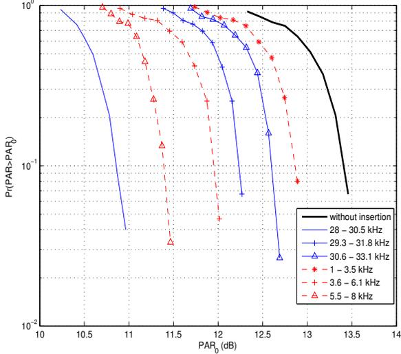
Fig. 3. CCDF of the PAR when control tones are inserted above the useful bandwidth (solid) and below the useful bandwidth (dashed). Legend indicates the bandwidth occupied by the control signal.
