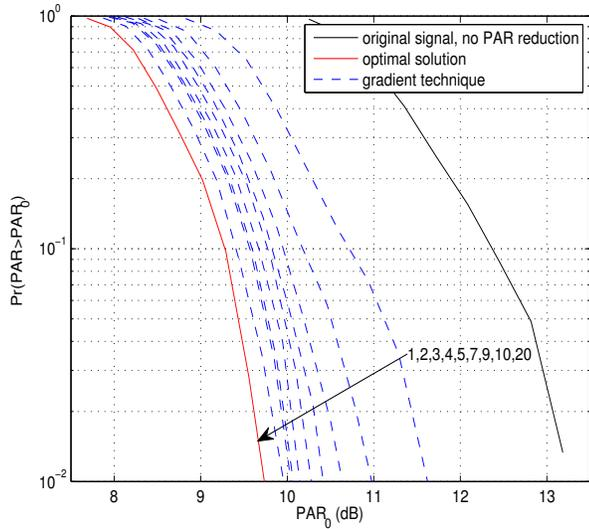
Fig. 6. CCDF of the PAR resulting from the gradient technique after a varying number of iterations.
