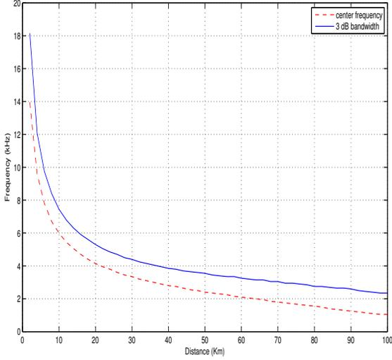
Fig. 1. Optimal center frequency and the 3 dB acoustic bandwidth as functions of distance (Stojanovic, 2006).
