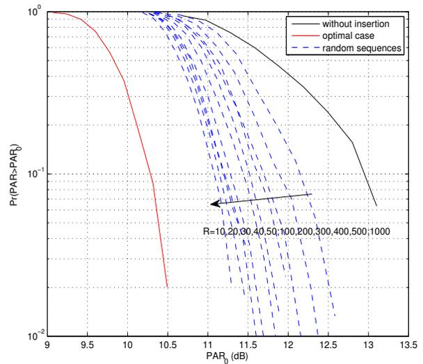
Fig. 9. CCDF of the PAR resulting from random insertion technique with a varying number of trials. The data and the control sequence are modulated using QPSK.
