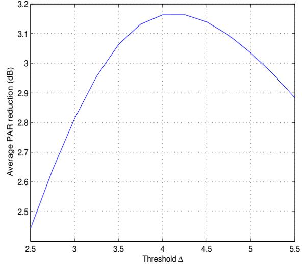
Fig. 5. Average PAR reduction as a function of the threshold  $\Delta$ .
