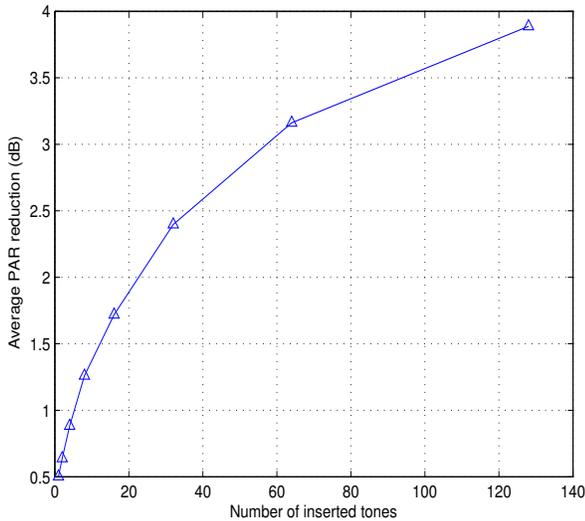
Fig. 4. PAR improvement vs. the number of out-of-band tones.
