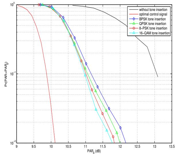
Fig. 8. CCDF of the PAR resulting from random insertion technique. The data sequence is modulated using QPSK, and the number of trials is limited to 100.
