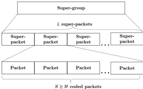
Figure 1. Grouping hierarchy of the proposed packet coding technique.
