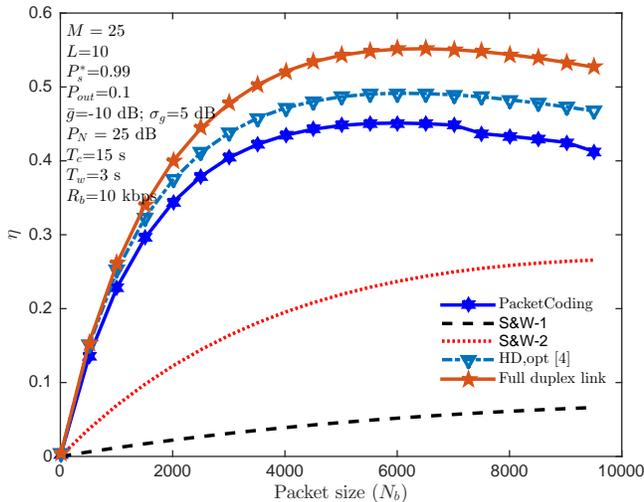
Figure 5. Throughput efficiency  $\eta$  as a function of the packet size  $N_b$ .
