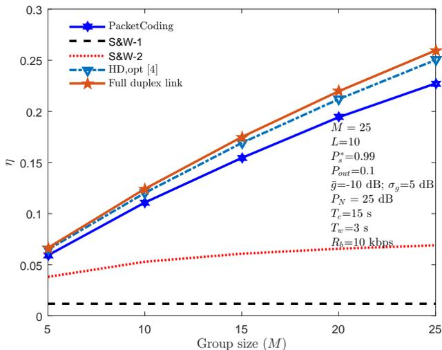
Figure 6. Throughput efficiency  $\eta$  as a function of the group size  $M$  under the assumption of log-normal distribution for the channel gain  $G$ .
