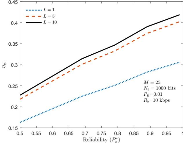
Figure 4. Throughput efficiency  $\eta$  as a function of the reliability  $P_s^*$ .
