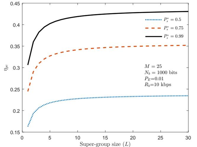
Figure 2. Throughput efficiency  $\eta$  as a function of the super-group size  $L$ .
