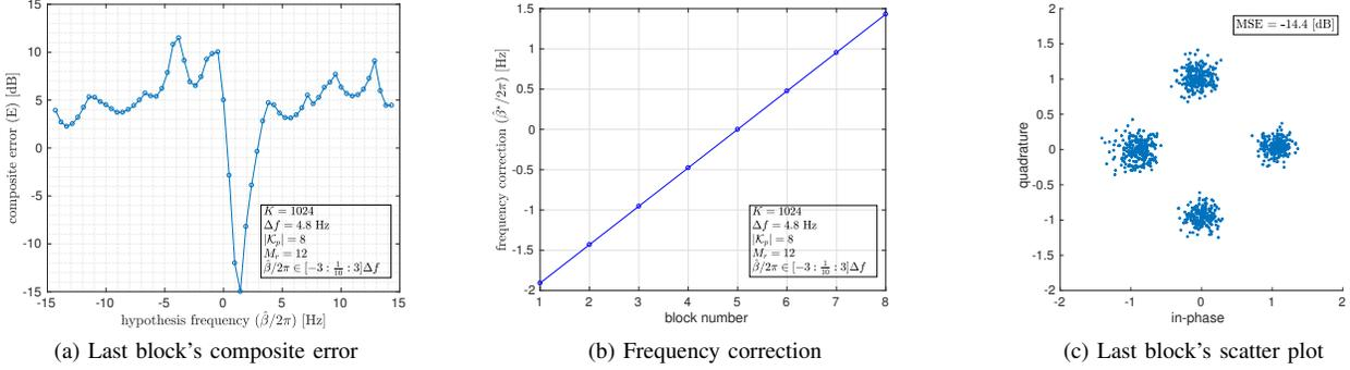
Fig. 1. Performance illustration for an OFDM frame with  $K = 1024$  carriers and 8 blocks. Shown are the composite error obtained for the last block (a), frequency correction (b), and the last block's scatter plot (c). Only 8 pilots are used and the hypothesized values range from  $-3\Delta f$  to  $3\Delta f$  in steps of  $\Delta f/10$ . There are no symbol decision errors in the scatter plot shown.
