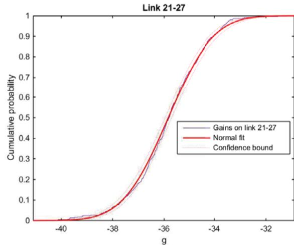
Figure 7. Cumulative distribution of the recorded gain  $g$  between nodes 21 and 27. The 95% confidence intervals and the normal distribution fit is also plotted.
