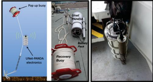
Figure 4. Unet-PANDA typical set-up.
