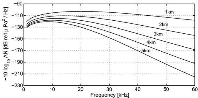
Fig. 1. Frequency-dependent part of the narrowband SNR in decibels,  $10 \log_{10} 1/(A(l, f)N(f))$ , for different transmission distances (attenuation constant  $A_0 = 30$  dB, spreading factor  $k = 1.5$ ).
