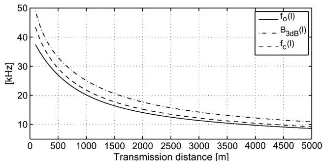
Fig. 2. Optimal frequency  $f_o(l)$ , 3-dB bandwidth  $B_{3\text{dB}}(l)$ , and center frequency  $f_c(l)$  (spreading factor  $k = 1.5$ ).
