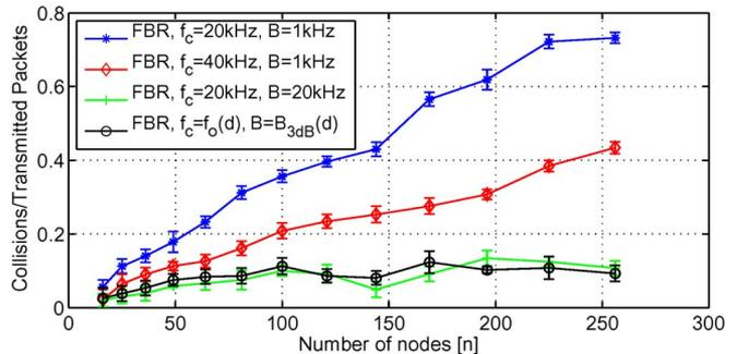
Fig. 11. Total number of collisions over transmitted packets for different frequency allocation patterns. Power control is implemented with four uniformly distributed power levels. The error bars represent the uncertainty interval at the 95% confidence level.
