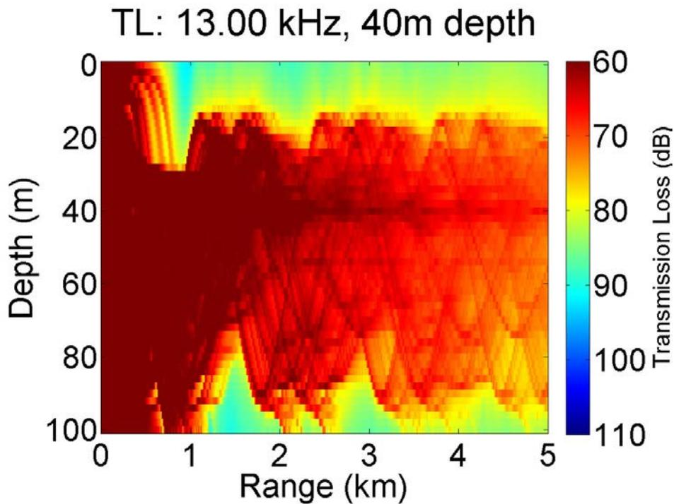
**Figure 3.** Transmission loss computed using the Bellhop model for the sound-speed profile observed during the MACE 2010 experiment.
