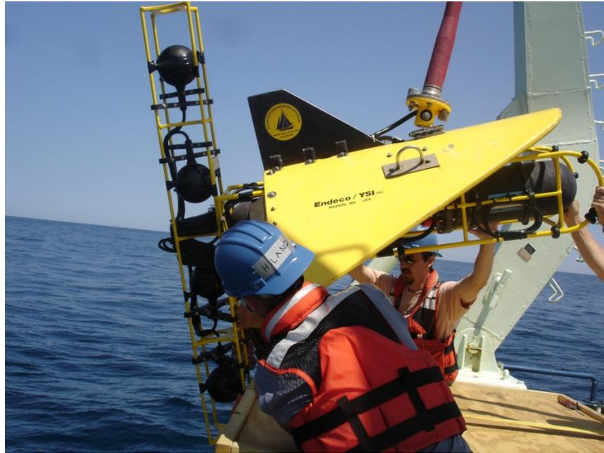
**Figure 1.** A tow fish with a four-element vertical source array is deployed on the *R/V Oceanus* during the MACE 2010 cruise south of Cape Cod, MA.
