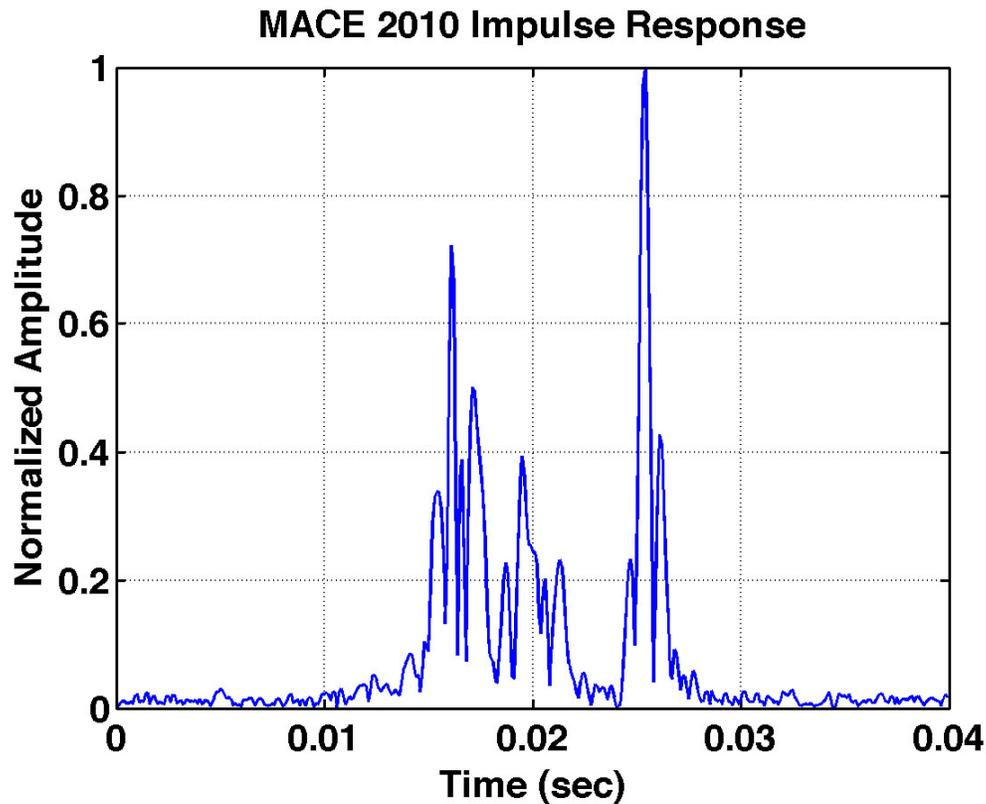
**Figure 2.** Multipath measured during the MACE 2010 experiment during one of the source tows.
