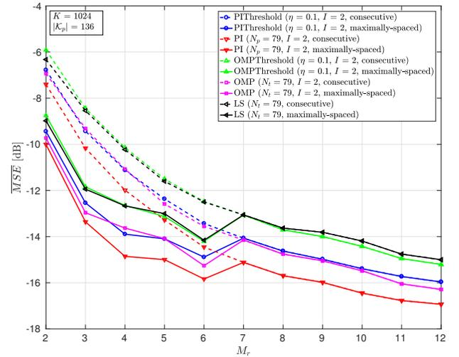
Fig. 4. Average MSE of the conventional LS, OMP and PI algorithms versus the number of receiving elements. The number of carriers and the resolution factor are 1024 and 2, respectively. For  $M_r \leq 6$ , two sets of receiving elements are chosen, one with consecutive elements and one with maximally-spaced elements.
