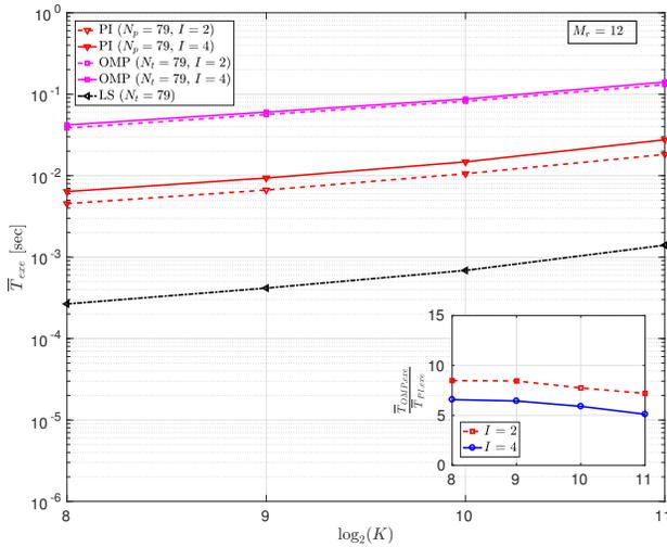
Fig. 2. Average execution time as a function of the number of carriers (log scale) and the resolution factor  $I = 2$  and 4. Execution time values represent the average over all blocks, 12 receive elements and 52 transmitted frames. The inset shows the ratio of the execution time of OMP algorithm to that of PI algorithm as a function of the number of carriers for  $I = 2, 4$ .
