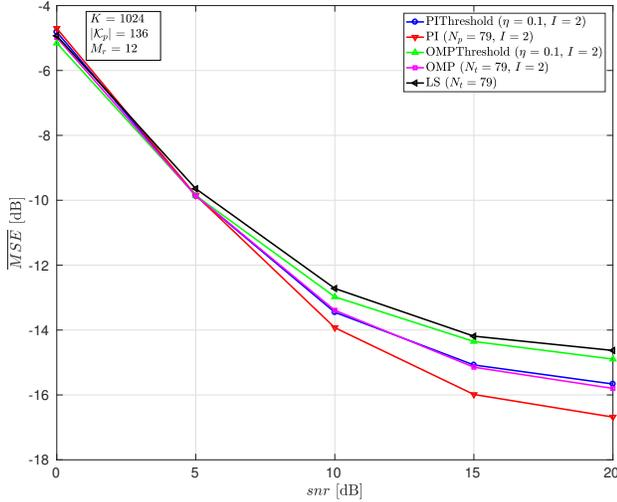
Fig. 5. Average MSE of the conventional LS, OMP and PI algorithms versus the input SNR. The number of carriers and the resolution factor are 1024 and 2, respectively. The number of receiver elements used to perform maximal ratio combining is  $M_r = 12$ .
