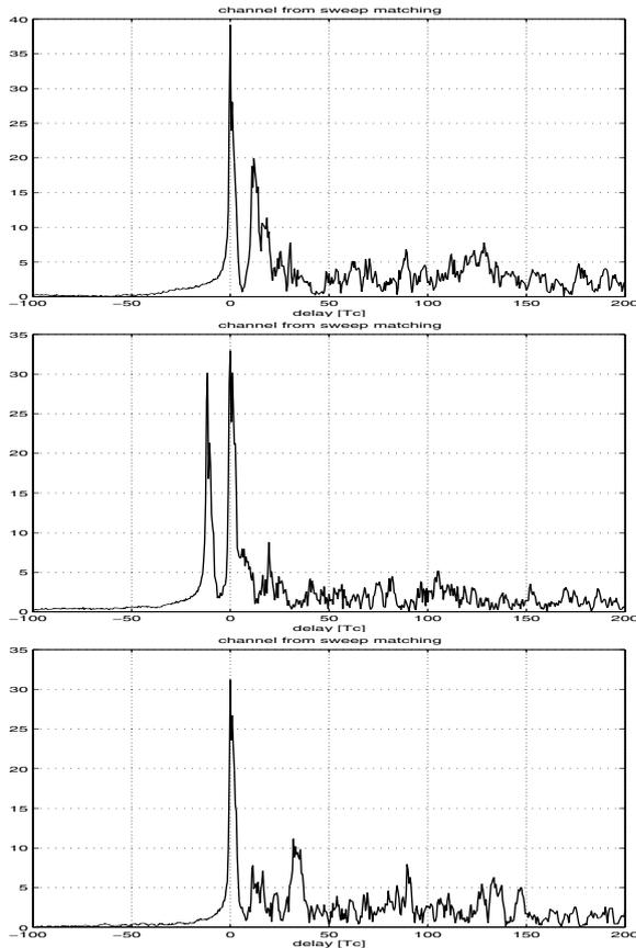
Fig. 1. Channel responses, estimated from the frequency sweep preamble prior to receiving the  $L=15$ , 63, and 255 group of multiuser signals (shown top to bottom, respectively).
