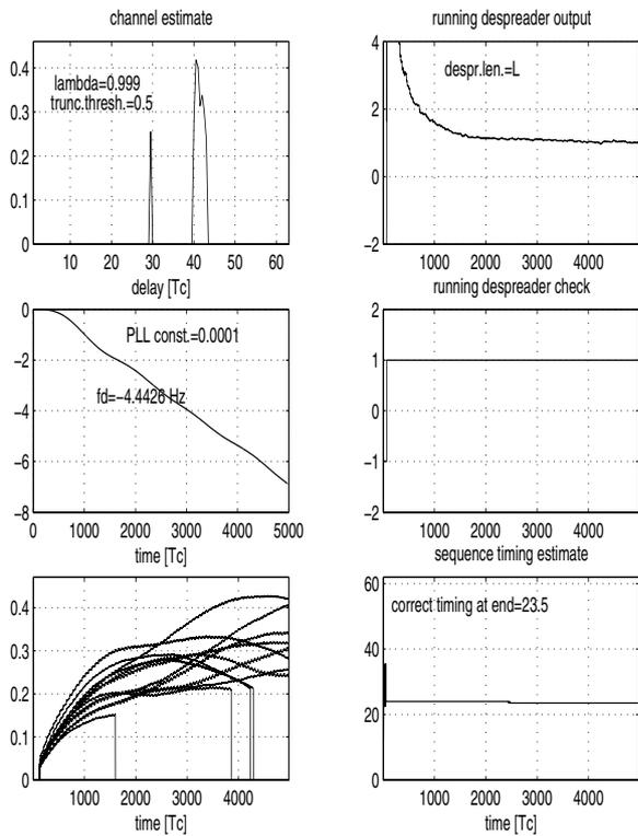
Fig. 3. Performance of the channel estimation and acquisition algorithm for a single-user, code length 63.
