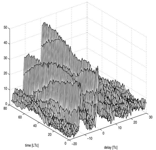
Fig. 2. Channel responses in time, estimated from the acquisition preamble. Each response represents cross-correlation between the received signal and one period of the spreading code.  $L=63$ , user #1.
