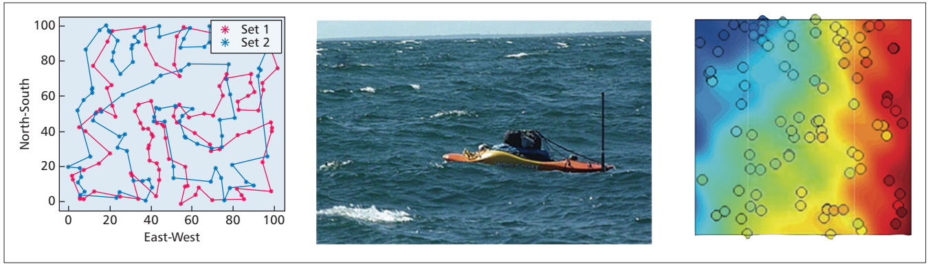
Figure 3. Kinematically-constrained sparse approximation in action at sea. The left image shows two “random TSP” paths generated and executed by an autonomous surface vehicle (center); the right image shows a depth-field reconstruction based on sparse samples and the discrete-cosine transform.
