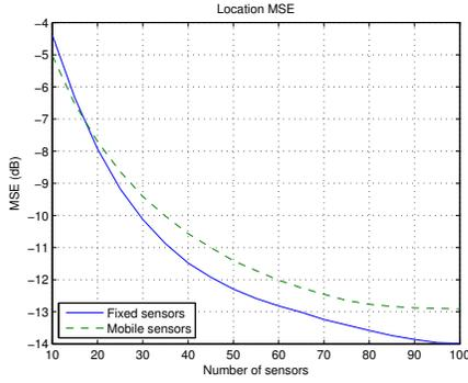
(a) Location MSE versus number of sensors with  $\alpha = 0.02 \text{ m}^{-1}$  and SNR= 0 dB
