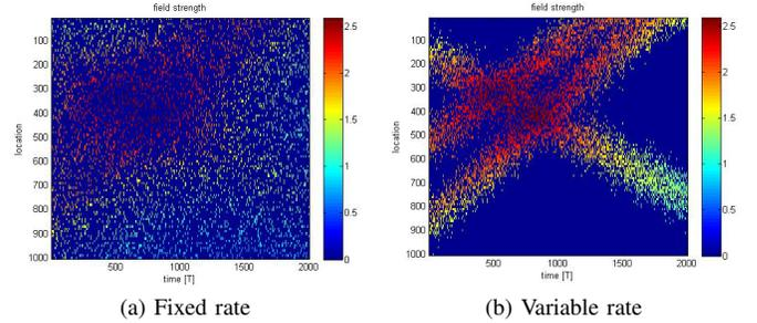
Fig. 1. Recovered field at the FC as it evolves across a one-dimensional track over time in a fixed-rate scenario and a variable-rate scenario. The length of the track is 1000 m and the number of sensors is 100. There are three objects with unit amplitude and a decay rate of  $0.002 \text{ m}^{-1}$ . The objects start at midpoints with velocities 3 m/s, -4 m/s and -5 m/s.
