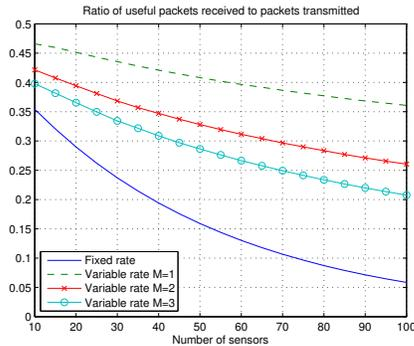
(c) Ratio of useful packets to packets transmitted
