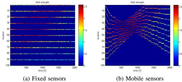
Fig. 2. Recovered field at the FC as it evolves across a one-dimensional track over time in a fixed-sensors scenario and a mobile-sensors scenario. The length of the track is 100 m and the number of sensors is 10. There are three objects with unit amplitude and a decay rate of  $0.002 \text{ m}^{-1}$ . The objects start at midpoints with velocities 0.3 m/s, -0.4 m/s and -0.5 m/s.
