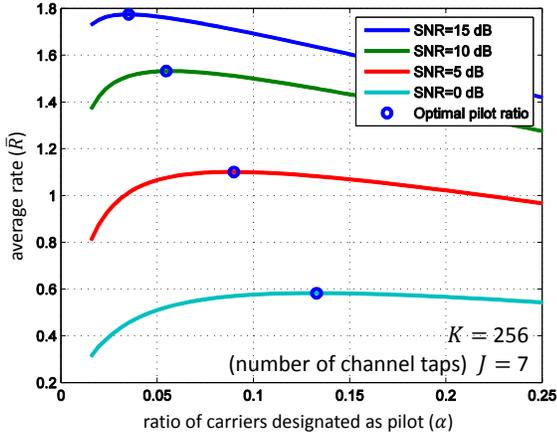
Fig. 1: The average rate (per channel use) for QPSK modulation depends on the ratio  $\alpha$  of carriers dedicated as pilots. With too few pilots, the receiver suffers from estimation errors, while assigning too many pilot carriers increases the pilot overhead. The best trade-off is marked with circles for each SNR value.
