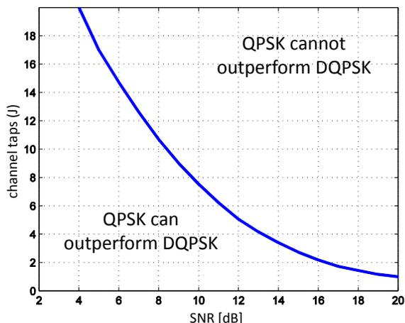
Fig. 4: Scenarios where DQPSK outperforms QPSK. Fig 3 shows that for any SNR, the performance of QPSK and DQPSK modulation cross as the number of channel taps grows. This figure visualizes the crossing point of the performance. If the channel statistics fall on the right hand side of this curve, DQPSK is the clearly the favorable choice as it deliver higher average rate at lower complexity.
