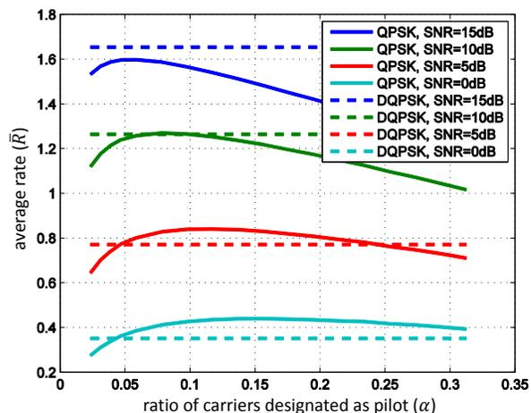
Fig. 6: Results from simulations with parameters taken from experimentally measured underwater acoustic channels. At SNRs higher than 10 dB, DQPSK outperforms QPSK in this simulation, suggesting that for high-SNR underwater acoustic channels, DQPSK is clearly the better choice when compared to QPSK.
