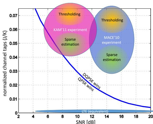
Fig. 5: Parameters of typical wireless and underwater acoustic channels. Although statistics of typical wireless channels do not fall into the region where DQPSK is the clear choice, but most underwater acoustic channels fall in this category.
