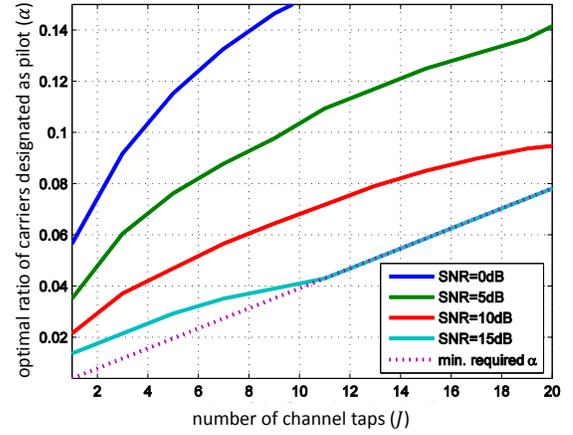
Fig. 2: Optimal ratio of pilot carriers as a function of channel taps. The optimal ratio of pilot carriers depends on the SNR and the number of channel taps. A larger ratio of carriers should be assigned as pilot when the channel has more taps, or when the SNR is low. Also note that at higher SNRs, the optimal number of pilot carriers is dictated by the channel estimation algorithm, which is shown by the dashed line.
